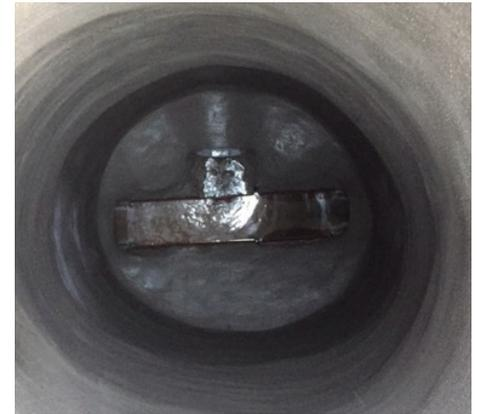
*GeoKrete Geopolymer showed no signs of cracking and peeling.*
