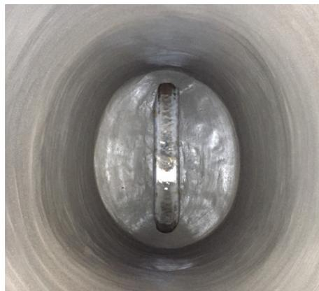
*GeoKrete Geopolymer showed no signs of cracking and peeling.*
